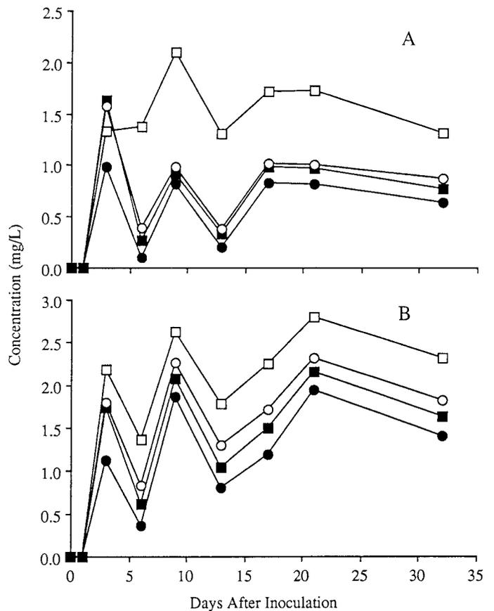
Fig. 8. Production of ethyl hexanoate (A), and ethyl octanoate (B) by *Saccharomyces cerevisiae* during fermentation. Juice fermented without insoluble material (□), with insoluble grape solids (■), with yeast ghosts (○), or with insoluble grape solids and yeast ghosts (●).
