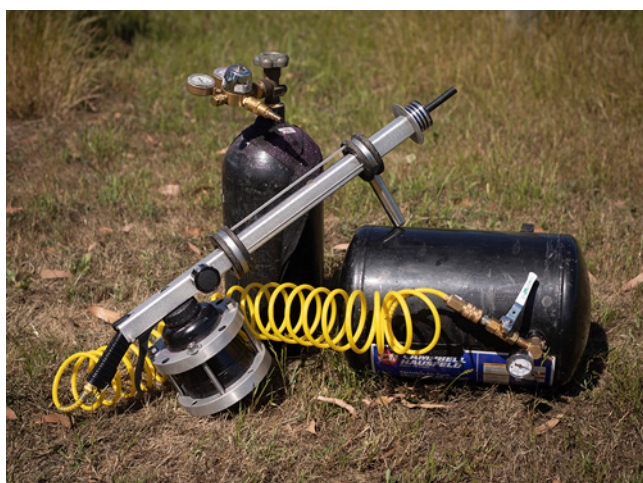
Figure 4 Yeast Blaster Prototype One applicator for dry addition of yeast for bioprotection. The unit includes a canister for holding dry product and two gas attachments in high-pressure and low-pressure serviceable systems. Backpack unit not shown.
