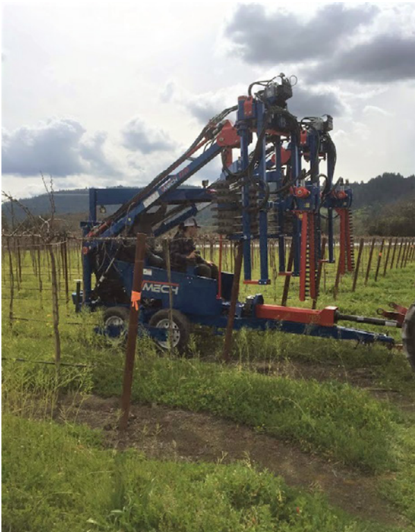
Figure 10 A rotary and drum mechanical pruner used in mechanical box pruning with hedger bar cutters on the side removing the sprawl.
