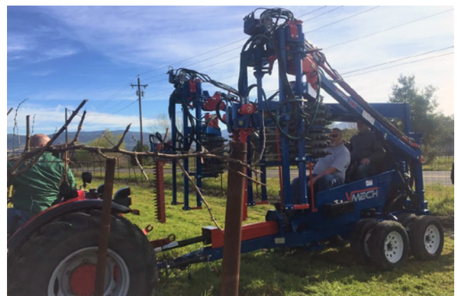
Figure 12 A multipurpose carrier frame with combination mechanical pruners installed that can prune two rows at a time in a Chardonnay vineyard in the central coast of California.
