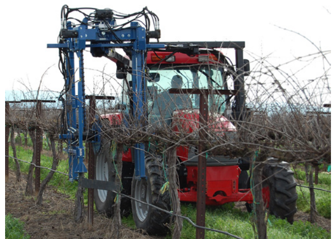
Figure 9 Hedger bars removing the sprawl and undergrowth of a sprawling canopy in Madera County, California.
