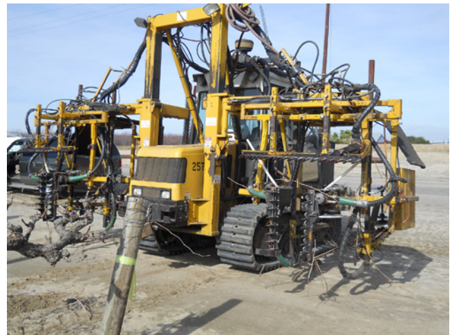
Figure 11 A combination mechanical pruner that is used in California sprawl type trellis in the San Joaquin Valley of California.
