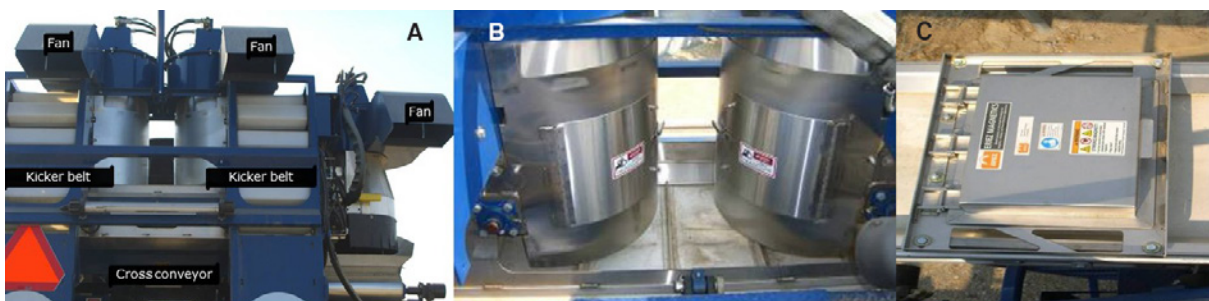
Figure 16 The cleaning system of a typical mechanical harvester indicating the location of (A) the kicker belt and cleaning fans, (B) the kicker belt and the drop cleaning fans, and (C) the ferrous material cleaner on the over-the-row conveyor before fruit is delivered to receptacle bin.
