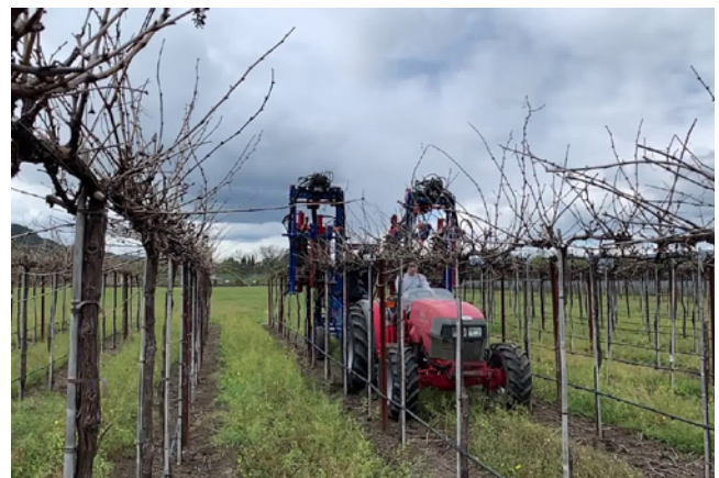
Figure 8 Mechanical prepruning at a Cabernet Sauvignon vineyard in Napa County, California.
