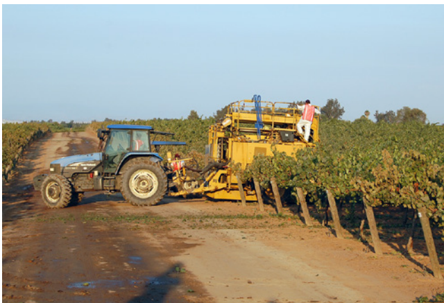
Figure 2 Proper spacing between alleyways will ensure long-machines can turn into rows easily.
