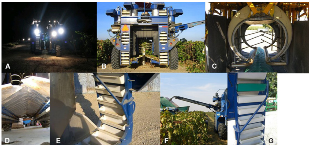
Figure 15 Parts of a mechanical harvester, typically used in California, operating (A) at night, with (B) a canopy shaker head with the bow rods visible, (C) a trunk shaker head with the rails in the bottom above the catcher plates, (D) the catcher plates that go around the trunk and line posts, (E) the conveyor belt with food grade buckets that transports the berries to the top of the harvester to the kicker belt, (F) the over-the-row conveyor used to deliver fruit to receptacle bin in the neighboring row, and (G) passive mechanism for keeping canes and sticks out of the fruit buckets with the slider bar.
