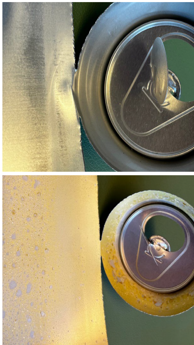
Figure 3 Representative images of cans scored with a “0” (top panel, undamaged BPA-epoxy) and “5” (bottom panel, badly damaged acrylic).
