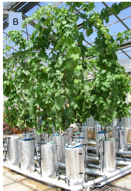
Figure 1 Schematic diagram of root-zone temperature treatment schedule in relation to developmental stage and measurement schedule ( A ), and the root-zone temperature control system and remaining vines just prior to the final destructive harvest at veraison ( B ).
